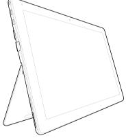
⚠ Important: Do not use excessive force when setting the kickstand angle or push down on the tablet when stood using the kickstand. This may damage the tablet and can cause the kickstand to stop working correctly.
